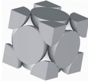
**Fig. 32: An *fcc* unit cell in the bulk.**
